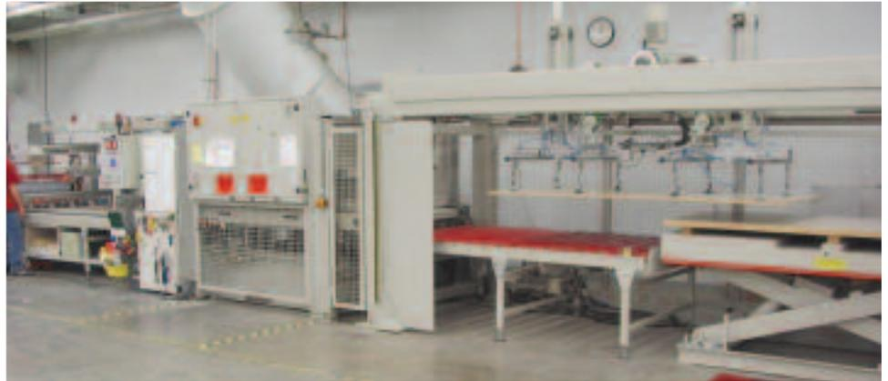
*Switching the manufacturing process from a cold press to a Joos throughfeed hot press and stacking line has saved A-dec considerable production time and increased profits.*
